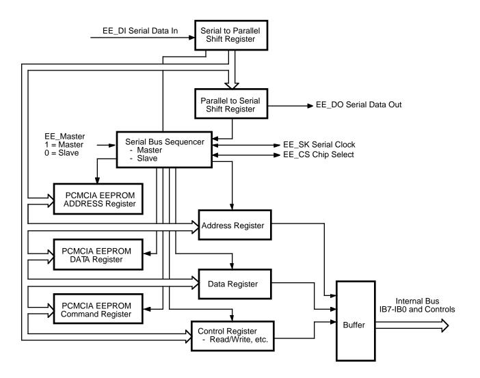
Figure 1-6. Serial Interface Diagram
