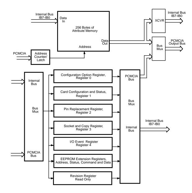
Figure 1-7. Attribute and Configuration Memory Diagram
